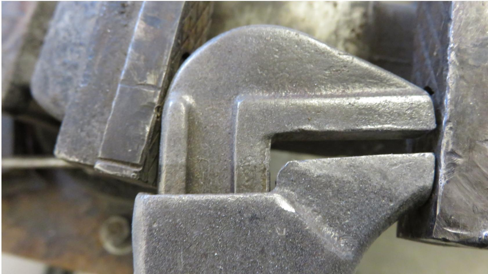
The jaw of my wrench had mushroomed because of abuse and soft steel metal. I hammered them flat while cold on an anvil. Put the jaws of the wrench in the vise so that the lower jaw end is parallel to the vise jaw face. Note that the fixed wrench jaw is not protected from the vise. I have ground the vice jaws down so they do not leave marks on whatever is held in the vice, you may need to use jaw protectors. The wrench needs to be open enough for the lower jaw to move closer to the upper jaw.
